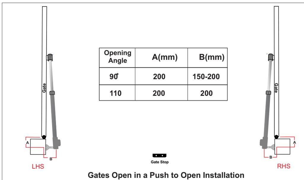
**1** Install the center of the post bracket in line with the center of your gates horizontal rail using the supplied dimensions above.
