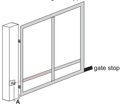
**Ensure you allow sufficient clearance for the motors fixing point on the post bracket to the floor.**
